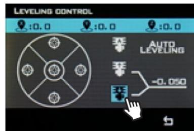
5. Adjust the height of the nozzle until it pinches the paper, checking each time whether the paper can be moved or not. Once the paper cannot be moved, return to the main menu and touch
